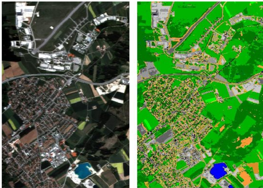
Figure 5.88: Example of classification with SPECL.
